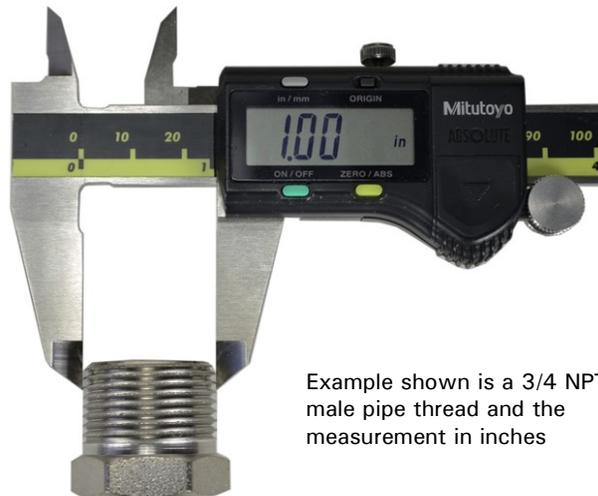
Example shown is a 3/4 NPT male pipe thread and the measurement in inches
