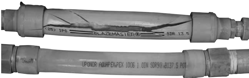
Figure 2-4: CPVC vs. PEX Freeze Test
