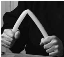
Figure 2-3: Reforming Kinked Piping
