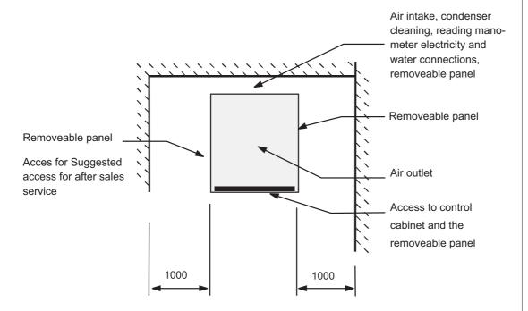
The distance from any constructions blocking the air supply must be at a minimum distance of 1 meter.
