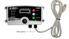
The empty gland on the left is for the power supply unit cable. A third gland must be fitted if the optional beacon is to be installed. Both of these cables must be fitted by the installer.
