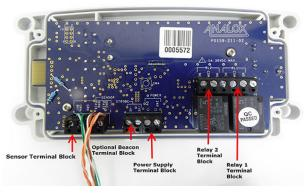
The Central Display's terminal blocks must be connected to the power supply, beacon and relays (the Sensor terminal block has a cable already fitted).
