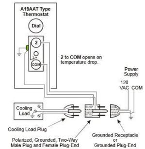
Figure 2: Wiring for the A19AAT Type Thermostat
