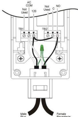
Figure 3: Factory Power Wiring
