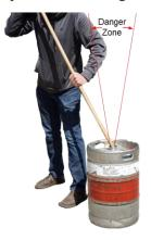
Be on the watch for any sign that a circlip is not fully seated in the keg neck. When discovered:
