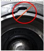
Always be on the lookout for **bent** or otherwise **damaged** circlips that may indicate **tampering** has occurred. Damaged circlips should be replaced by a trained technician before the keg is washed or filled again.
