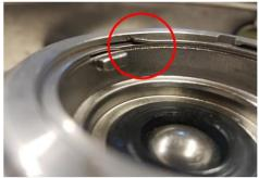
Look for signs of damage caused by forcing a circlip into place with a punch, screwdriver or pliers.
