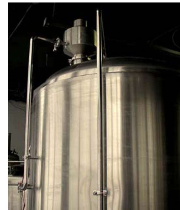
Hydrator at the top of Mash / Lauter Tun.
