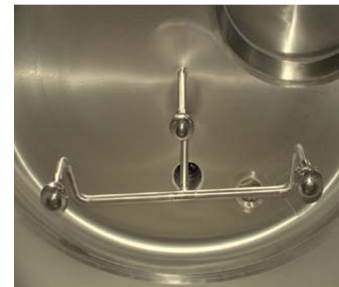
CIP Spray ball and sparging spray head.
