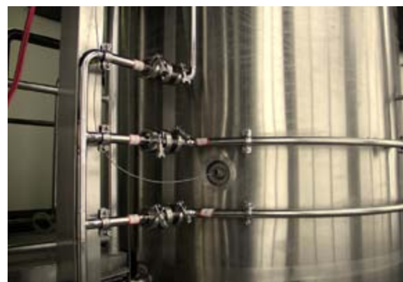
Temperature probe installed in Mash / Lauter Tun.
